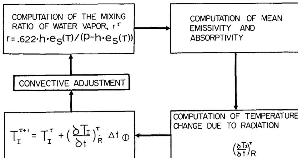
FIG. 2. Flow chart for the numerical time integration.
